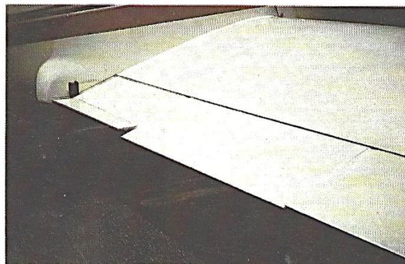
The right side flettner trim tab on the flap: upside deflection means downward force on flap and consequently nose up tendency of the airplane. Right and left side trim tabs are independently operated by two levers on the left hand side of the pilot.
