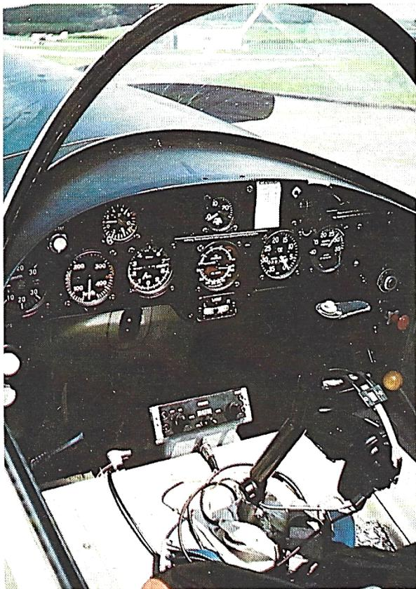
The Acrostar panel: in the center fuel and oil pressure gauges. On the right side manifold pressure and rpm indicator, on the left airspeed and altimeter, climb/descend and G-meter. Most indicators are metric. Throttle and rpm levers are left, mixer and manual fuel pump right.
