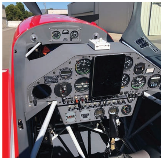
The Bolder Flight Systems OnFlight Hub data unit is simple, light, self-contained, and compact, requiring no modification on any aircraft. In this example, the unit is stuck with dual lock Velcro to the glare shield of an Extra 300L.
