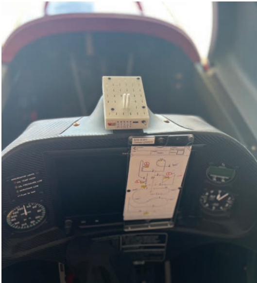
OnFlight Data Unit above the panel.
