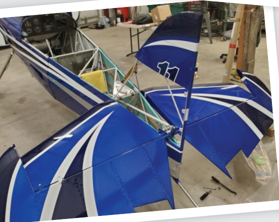
TOP: Modified wings with outer one-third swept leading edges and tapered spars with carbon wingtips.
