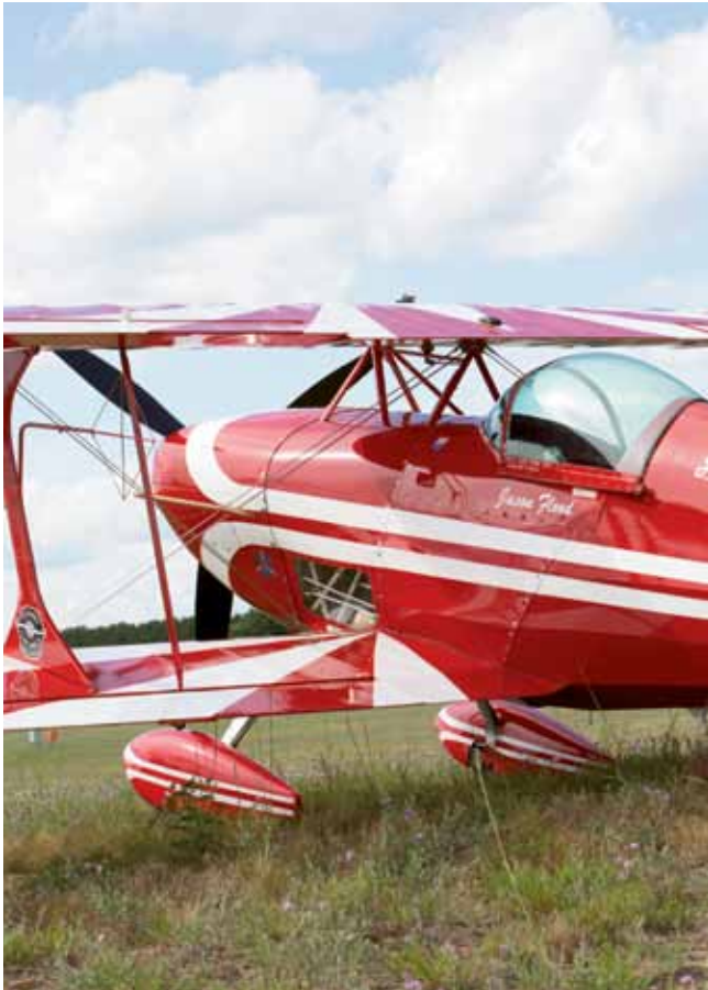
Spring gear replaces the standard steel tube and bungee arrangement of the original.
