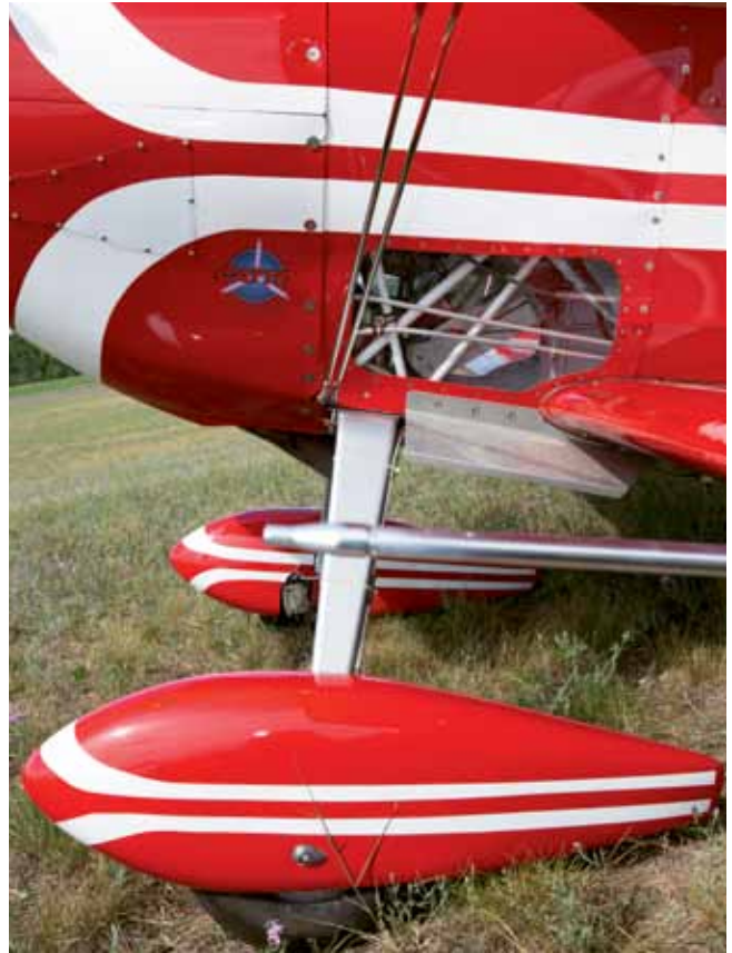
Spring gear replaces the standard steel tube and bungee arrangement of the original.
