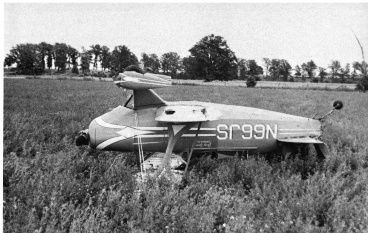
The result of the failure of a 25c pin in the fuel pump of Jerry Spear's Pitts.
