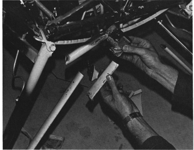
The relationship of the sections of failed tubing on the right gear leg.
