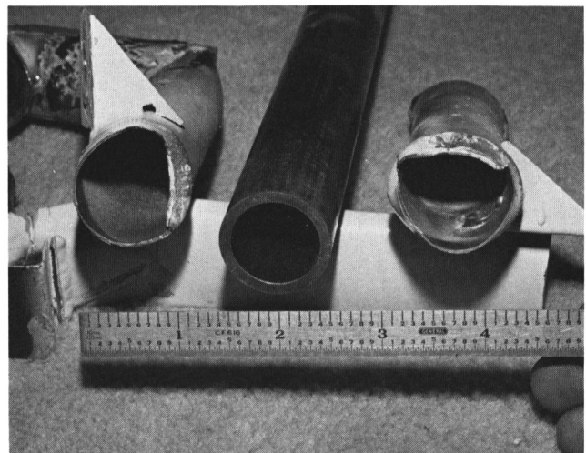
Dramatic illustration of the difference between the early 1.125" x .049 tubing (showing both ends of the failed section) and the later 1.250" x .120 tubing which replaces the same gear member.
