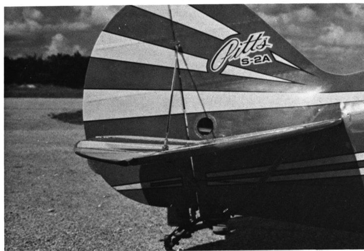
This was all the up-elevator available, with the control jammed in the S-2.
