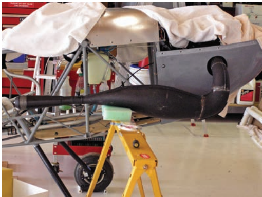
ABOVE: The tuned exhaust was very challenging to install correctly. RIGHT: The wing and fuselage are checked for fit.
