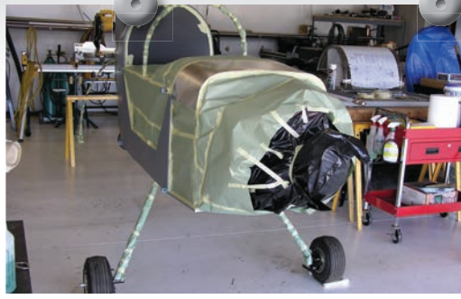
LEFT: Green glue binds the fabric to the fuselage. RIGHT: The Fuselage is masked and ready for paint.
