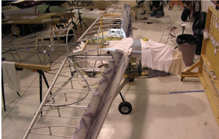
RIGHT: The left wing with fuel tank and wing walk ready for installation.
