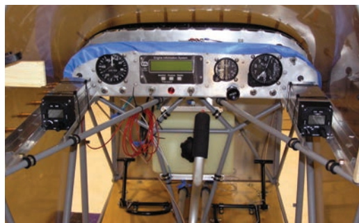
The instrument panel is seven inches further aft for accessibility in flight and ease of maintenance.
