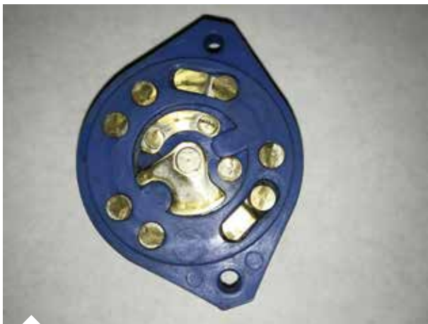
ACS contact plate with wear at 450 hours.
