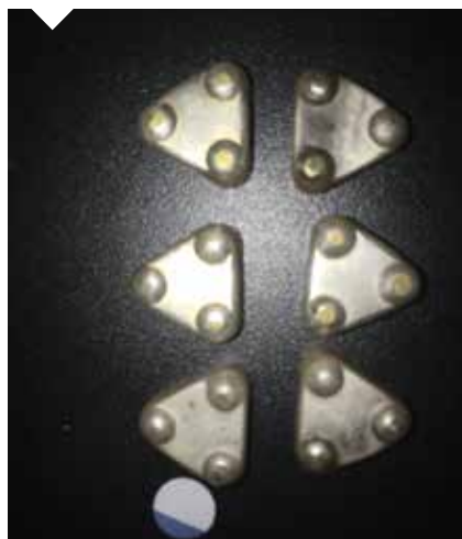
Switch contacts with various stages of wear. All rejected for service.
