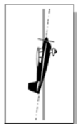
Figure 3. Vertical lines judged on attitude of the zero-lift axis, not the "apparent" longitudinal axis.
