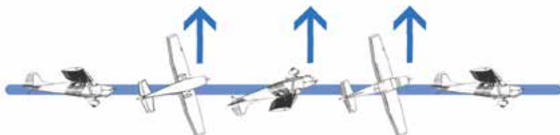
Figure 10. Slow Roll – beginning of roll is the key: Aileron roll – pitch first. Slow roll – “top” or “sky” rudder, then a “push” is used in place of the pitch up to keep aircraft from descending.
