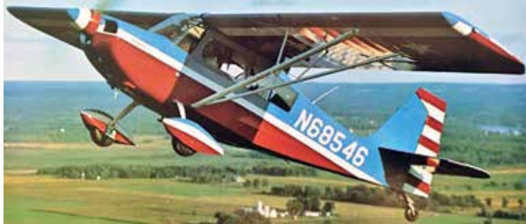
1970 Champion 8KCAB Decathlon prototype (symmetrical wing/150-hp/constant-speed prop).
