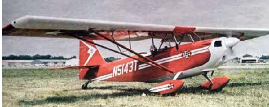
One-of-a-kind 1968 Champion Pro (symmetrical wing/180-hp/constant-speed prop).
