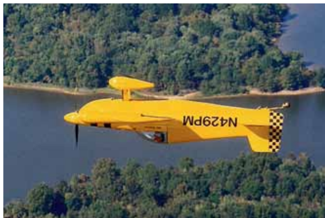
The Cassutt flies as well inverted as upright with full inverted fuel and oil systems.
