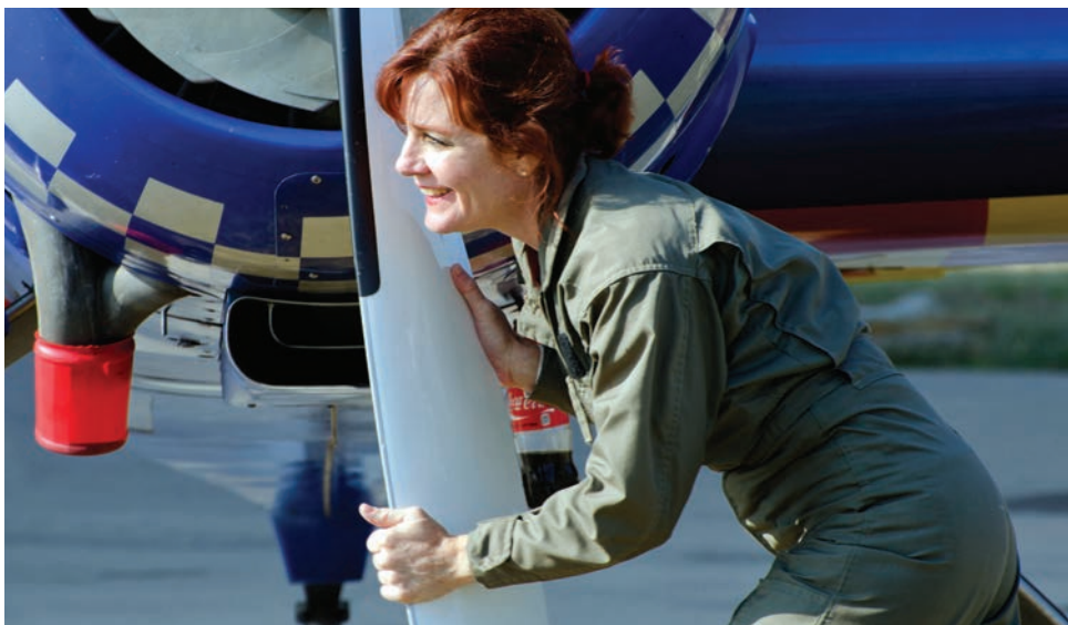
Twenty-one blades before start-up ensures no oil in the bottom cylinders.
