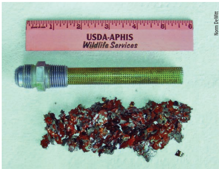
ABOVE: The oil sump showing the red paint. RIGHT: Paint chips removed from the finger screen.
