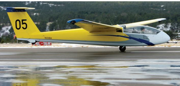
Gliders require aileron input to maintain wings-level during the takeoff roll.
