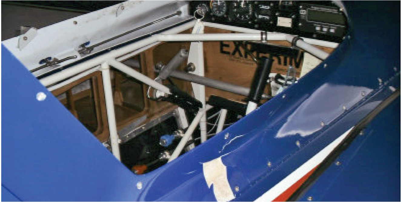
Detail shot of the damaged canopy hinging.
