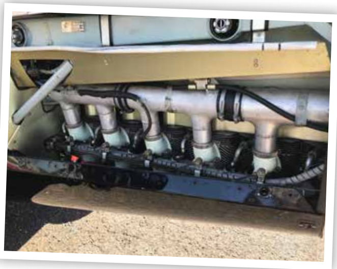
The Walter Minor six-cylinder air-cooled inverted in-line piston engine.
