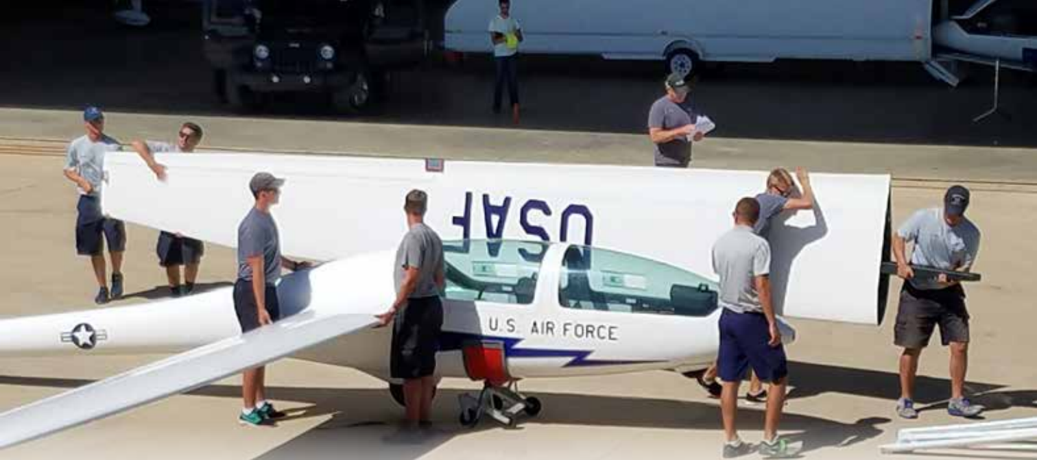
Cadets trailer their gliders to contest locations. Once at the contest site the cadets coordinate and stay focused to avoid missed steps. A critical assembly checklist is completed to ensure proper assembly has been completed.
