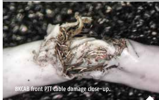
8KCAB front PTT cable and tubing damage.
