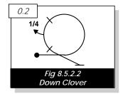
For the Family 0.2 quarter-clover, the first half loop up is like the first half of a 7.4.1.1. Immediately upon completing the first half loop, the aircraft must begin a constant rate quarter roll such as to reach upright, wings-level horizontal flight at the bottom of the second half loop.
