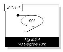
As soon as the aircraft is on the exit heading, the heading change must stop while maintaining the chosen bank angle, followed immediately by a roll back to wings level using a rate of roll equal to the entry roll.
