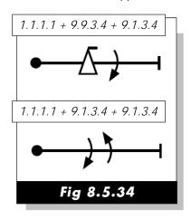
The pilot may elect to fly the first roll in either direction, but the second roll must be opposite direction to the first. Opposite rolls must have a brief pause between them, but long enough that the judge can discern each roll separately. If two unlinked rolls are of the same type, they must be flown in opposite directions.
