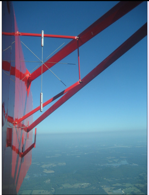
View on the Up Line. The pilot in the front cockpit puts the sight gage on horizon to guarantee the aircraft is vertical and to keep the wing tips level
